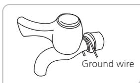
Connect the wire to metal pipe [no PVC pipe]
