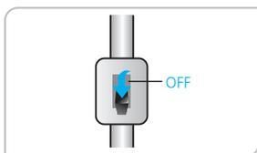
Equip earth leakage breaker and make sure to ground the wire to avoid an electrical accident
