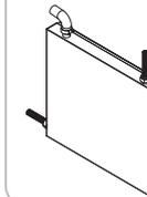
E/S device recovers the waste heat from drain water by heat-conduction. It makes washing capacity improving by reducing the energy consumption, heating time.
