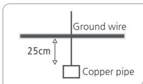
Connect the wire to Copper pipe
